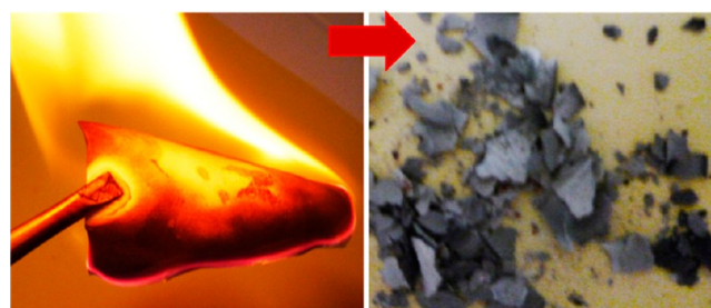
Figure 7. Representative image showing the possibility to incinerate the SH paper substrates up to an ash residue.
